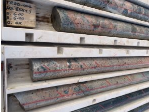
Core sample from drill hole TRDD002 at the Trundle Park target showing Potassic altered monzonite porphyry with chalcopyrite-chlorite clots. Photo Credit: Kincora Copper.
